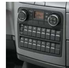
Controls for the air-conditioner, heater and ventilation. Switch panel with function displays.
