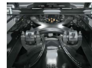
Weight-optimised X control arm with stabiliser and control arm function for semitrailer tractors and high-load roll stabilisation for 6x2 vehicles.
