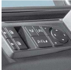
Ergonomically styled door control module for locking, mirror adjustment and window lifters.
